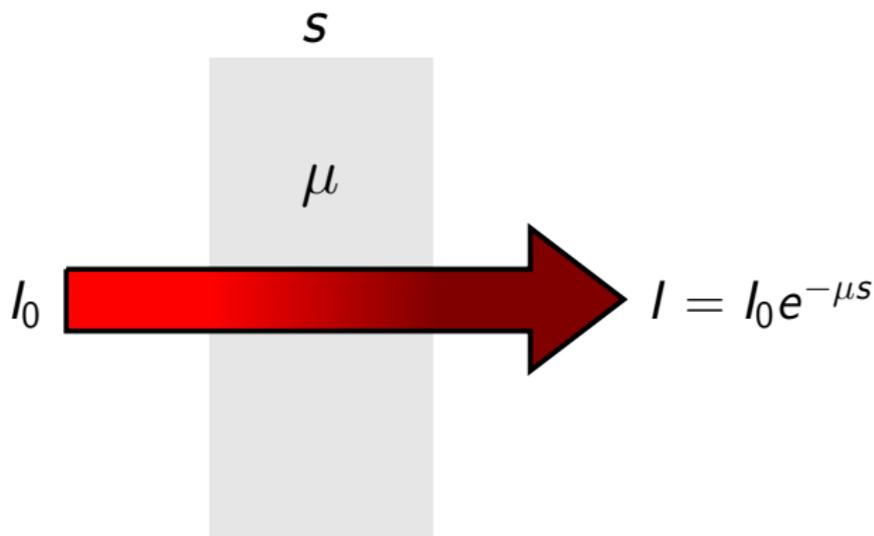
Here  $s$  is the thickness of the homogeneous medium and  $\mu$  is the *linear attenuation coefficient*.
