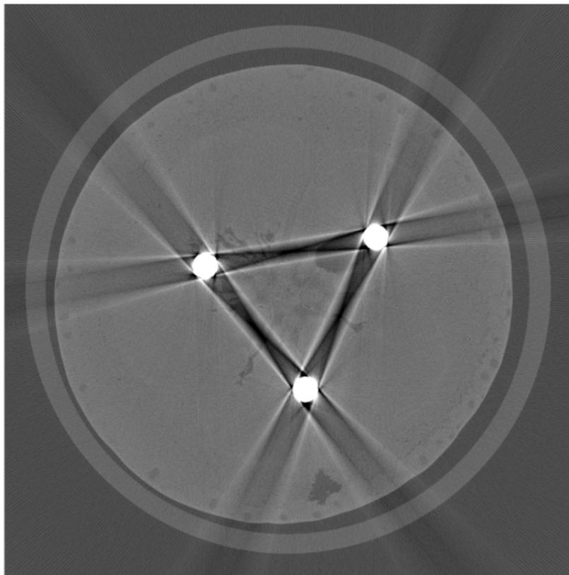
Metal artefacts in kumquat fruit with three inserted steel nails.
